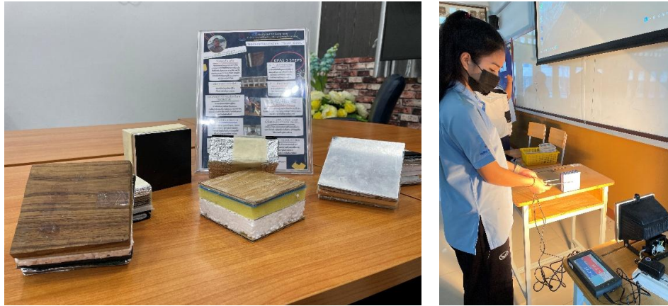
Figure 4 Student-designed thermal insulation prototypes (A) and an in-class test of heat insulation performance using a heat lamp and temperature sensor (B).
